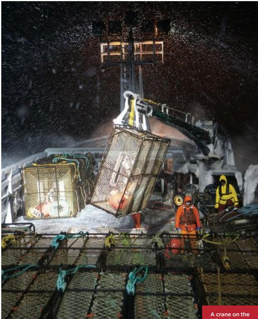
A crane on the Wizard moves 1,000-pound crab pots in three-story seas and 65-mph winds. Equipment failure and rogue 50-pound blocks of frozen spray flying on deck can easily kill a man.
